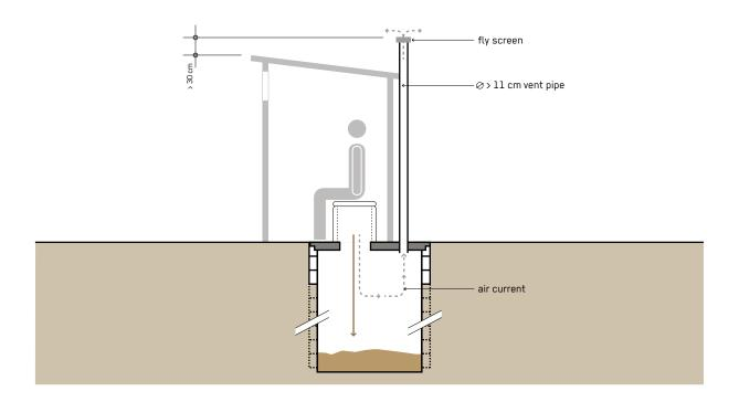
The Single VIP is seen as an improvement over the Single Pit Latrine (S.3) because continuous airflow through the ventilation pipe prevents odours and acts as a trap for flies as they escape towards the light.
